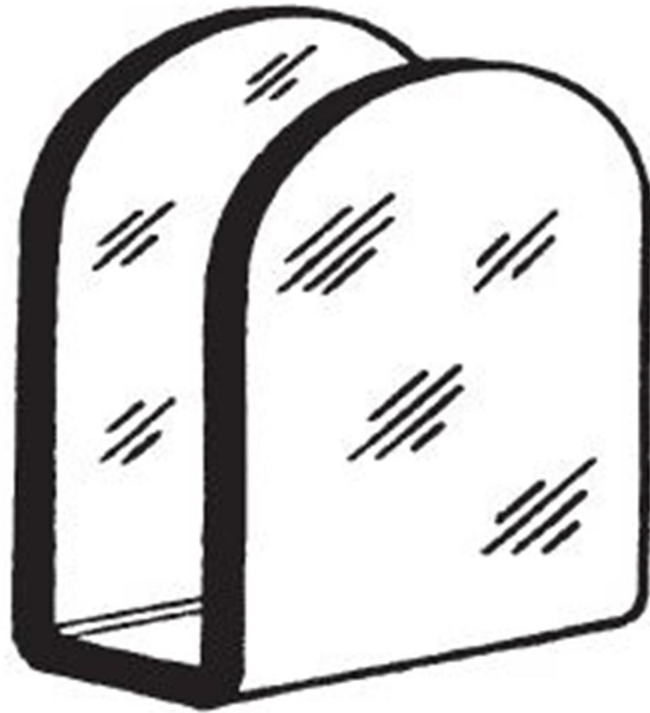
Figure 1.34 Stamping bent in a bending die.
