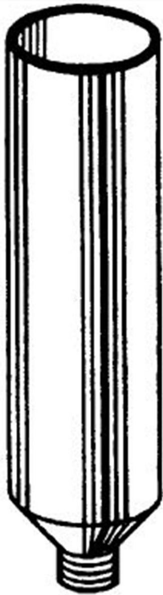
Figure 1.40 Drawn shell that has been extruded.
