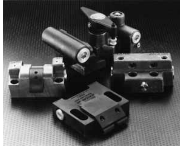
Figure 15-5 These hydraulic clamps are made with an internal locking device that mechanically locks the clamps against the workpiece when the power source is removed (Courtesy of Jergens, Inc.).
