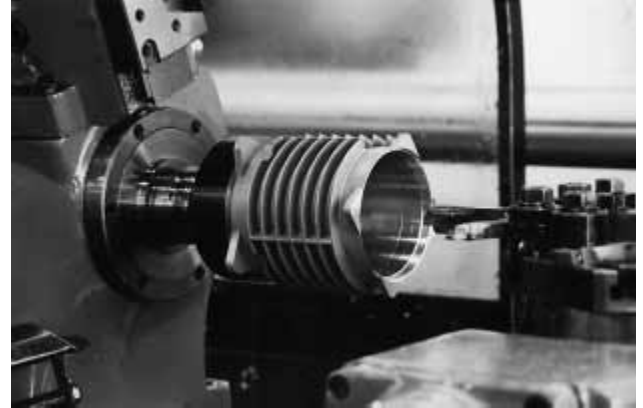
Figure 18-31 Expanding collet setup for boring a large-diameter workpiece (Courtesy of ROVI Products).
