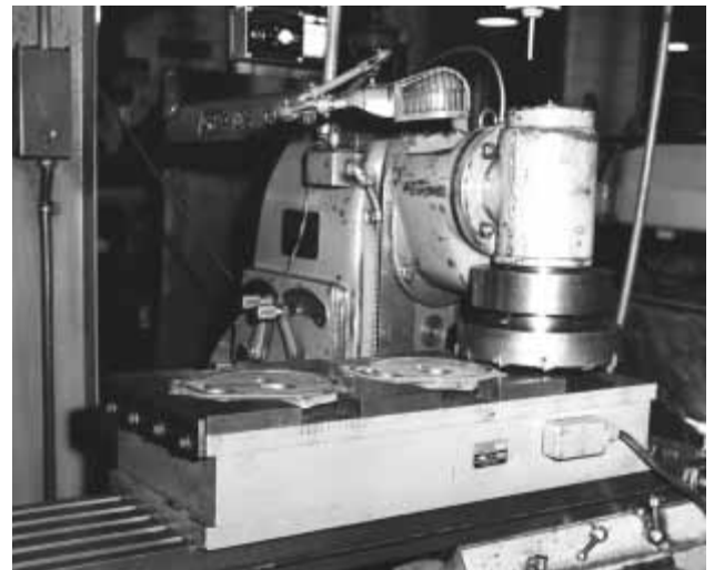
Figure 4-41 Machined packing elements made to conform to the complete outer shape of the workpiece.
