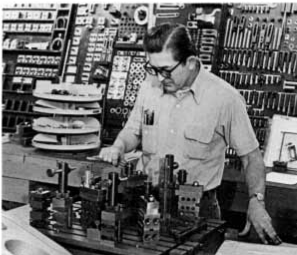
Figure 16-23 Constructing a modular workholder.
