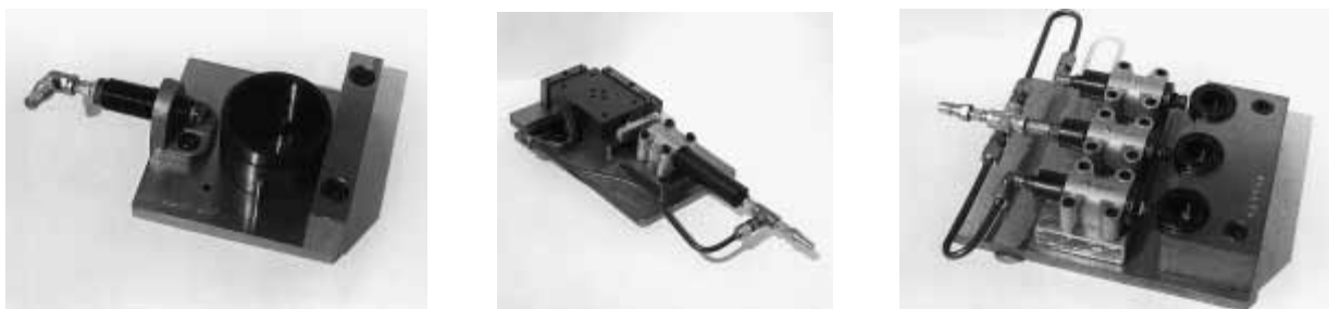
Figure 15–9 Typical applications of power clamping (Courtesy of Vlier Engineering).
