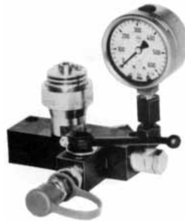
Figure 15-4 A pallet-decoupler unit uses an accumulator charged with either fluid or gas to maintain hydraulic pressure when the power source is removed (Courtesy of Carr Lane Manufacturing Company).
