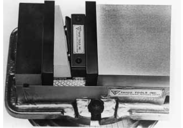
Figure 18-47 Odd and irregular parts are easily held with the Swivel Jaw™ vise accessory (Courtesy of TAYCO Tools, Inc.).
