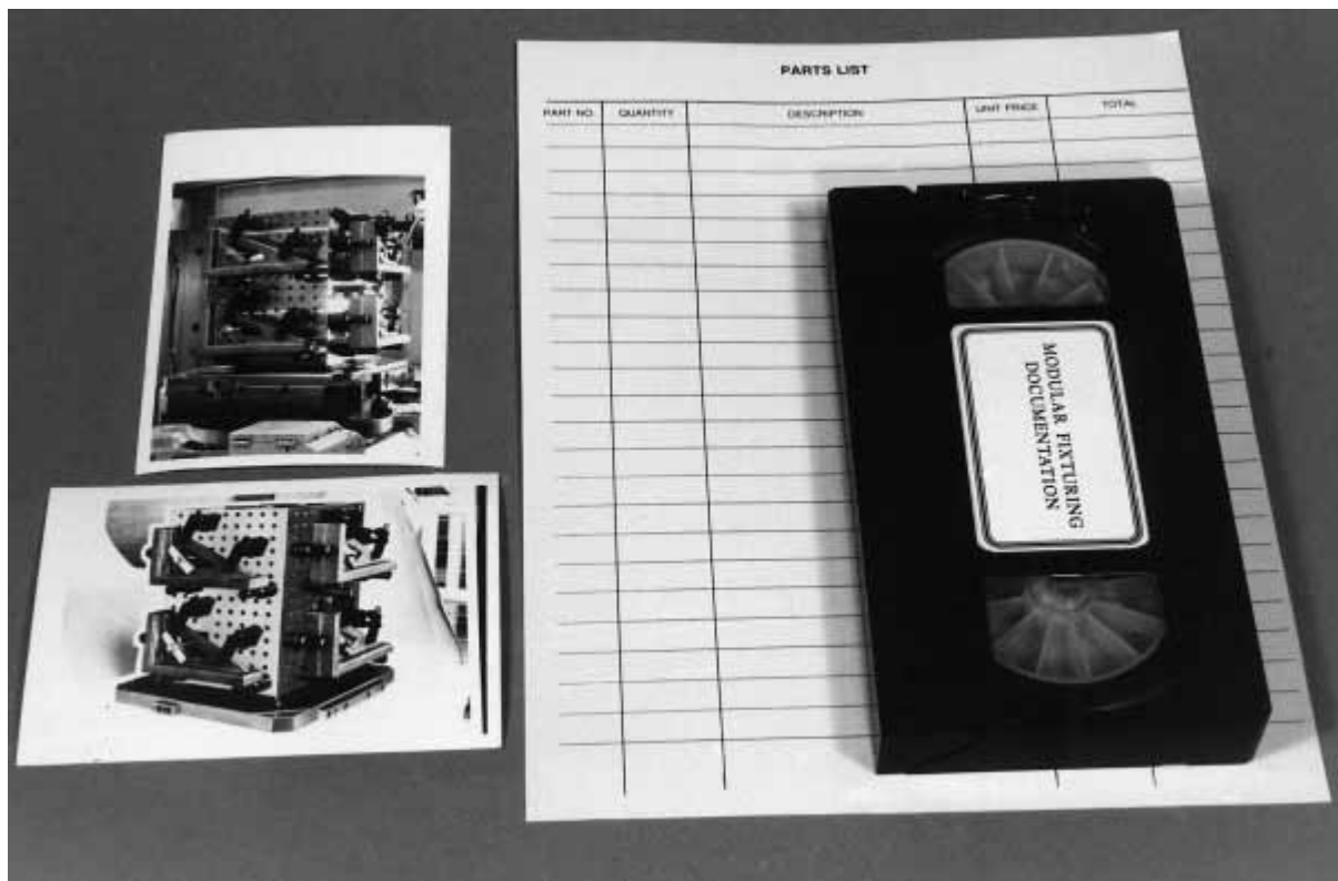
Figure 16–26 Once assembled, the fixture should be photographed or videotaped and the components noted on a parts list to keep a record of the workholder (Courtesy of Carr Lane Manufacturing Company).
