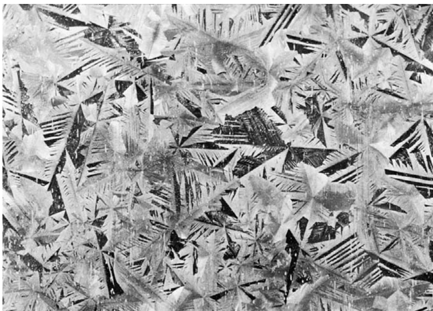
Figure 21.13. Spangles on the surface of a steel sheet that was hot-dip galvanized. From Making, Shaping and Treating of Steel, 9th Ed (1971) United States Steel Corp.
