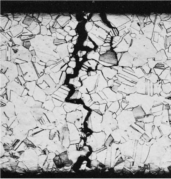
Figure 21.21. Stress-corrosion cracking in brass. From Metals Handbook , 8th ed. v. 7 ASM 1972.
