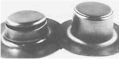
Figure 15.2. Drawing failures by necking at the bottom of the cup wall. From D. J. Meuleman, PhD thesis , University of Michigan (1980).
