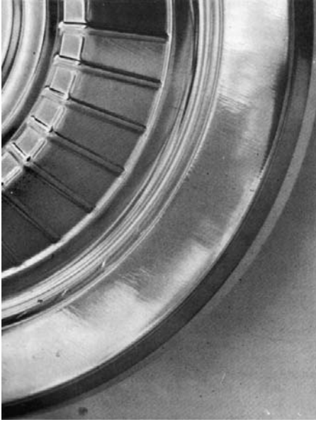
Figure 21.2. Ridging in a 430 stainless steel. From Making, Shaping and Treating Steels , 9th ed. United States Steel Corp. 1971.
