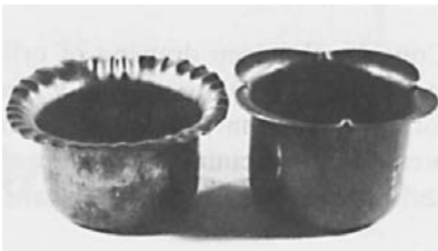
Figure 15.3. Wrinkling of partially drawn cups due to insufficient hold-down. From D. J. Meuleman, ibid.
