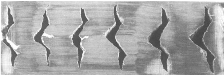
Figure 11.16. Cracks formed in a molybdenum bar during rolling under high \Delta conditions.
